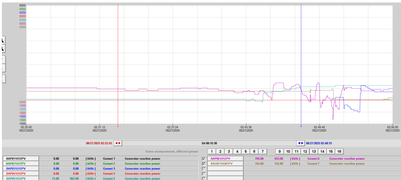
Reactive power Dokweg 1 units during last 30 minutes before blackout
