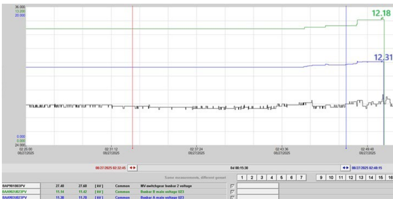
Busbar voltages Dokweg 1, 2A, 2B (black=DKW 1, green=DKW2A, blue=DKW2B)
